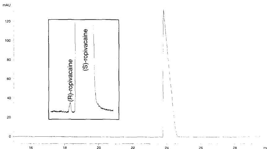
Fig. 3. LOQ for ( R )-ropivacaine in ropivacaine hydrochloride injection solution. Conditions as described in Section 2.
